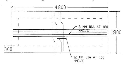
Thickness of slab = 100 mm All the covers = 20 mm
